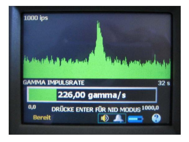
Screenshot of "Locator Mode" Search for a gamma source X-axis: time line Y-axis: gamma intensity Bar below: current gamma intensity
